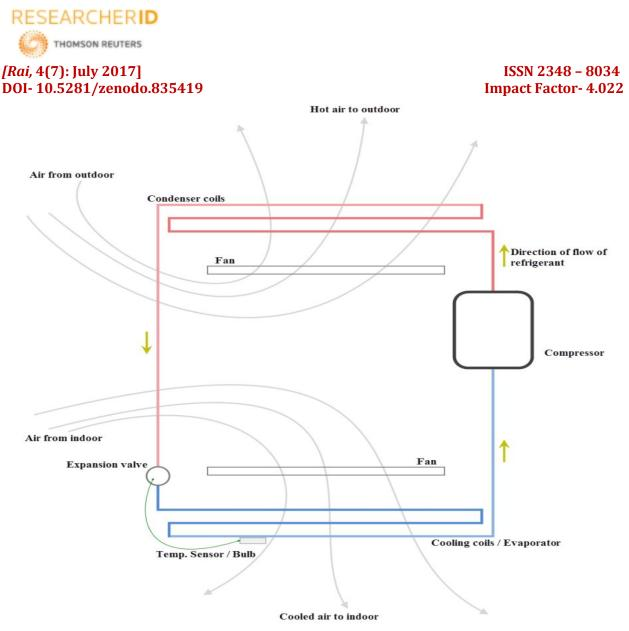
Fig [1] – Simple Air conditioner mechanism
