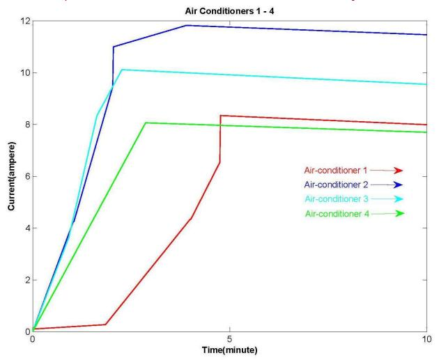
Fig [3] – Current and Time graph of air-conditioners in cold load pickup condition
